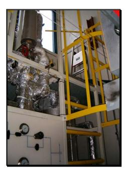
When a catalyst with the desired activity is identified from the screening study with help of the catalytic basket, its performance is then validated in a fixed bed reactor.
