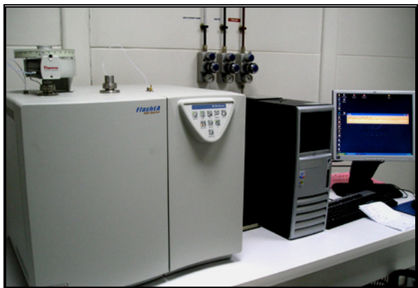
Organic Elemental Analyzer used for determining the chemical composition of organic compounds (C,H,N,O,S)
